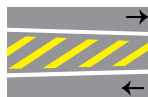
Channelizing island (do not drive over the marking except in an emergency)
