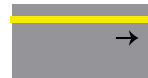
Left Edge Line On one way roads the right edge line is white
